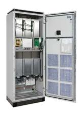
The **VERICON**® Active Harmonic Filter AHF is a new type of power electronic device for dynamically eliminating harmonics and compensating reactive power. It can compensate for the harmonic of varying magnitude & frequency and constantly changing reactive power in real time.
